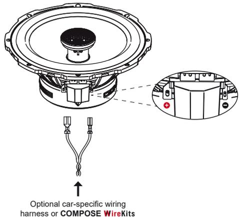
Ensure that all components are correctly connected (phase), i.e. plus to plus and minus to minus.
