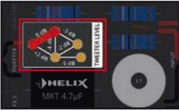
The crossover allows to optimize the level of the connected tweeter internally by repositioning the tweeter level jumper. Therefore open the crossover housing, pull the jumper straight upwards and reinsert it to the desired position.
