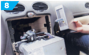
Connect S810 harness to headunit wiring harness
