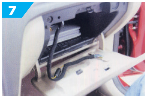
Pull through S810 wiring harness to installation location
