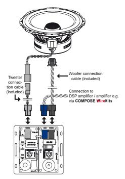
Option b: Universal connection to the tweeter connector and blade terminals via optional car-specific harness or COMPOSE WireKits, e.g. in active applications
