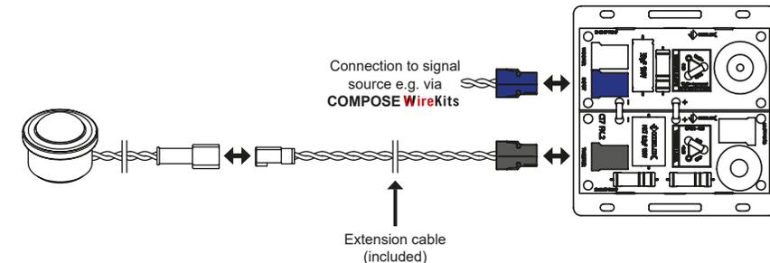
Ensure that all components are correctly connected in polarity, i.e. plus to plus and minus to minus. The positive leads of the loudspeaker system are marked red.
