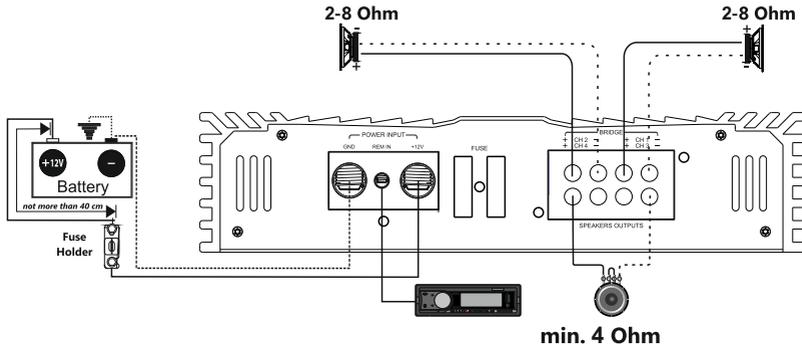
**Caution!!!** The minimum permissible connection load impedance at single channel is 2 ohm.
