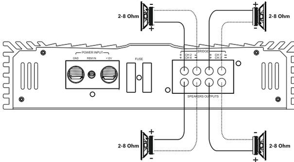
**Caution!!! The minimum permissible connection load impedance at single channel is 2 ohm. For amplifiers MLA-4080, MLA-4120 the operating voltage is 10-15 V.**
