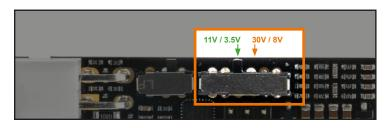
The factory setting of the input sensitivity (11 V / 3.5 V) of the module is appropriate for the most common radios.
