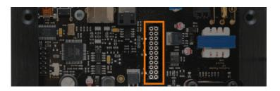
Make sure that the module is installed properly and all pins are fully inserted into the socket:
