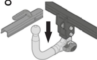
✓ Each time you install the towball into the socket, you must ensure that you can see the green field on the towball handle (3) and apply additional physical force to ensure that the towball is securely fastened in the socket. (6)
